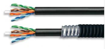
Aluminum Interlock Armor with Sunlight and Weather Resistant Polyethylene Outer Jacket (optional) Solid Annealed Copper Conductor Cross-web Separator (CAT 6 only) PFM<sup>TM</sup> Gel-filled, Water-Repellent Core Thermoplastic Insulation
