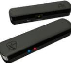
The DBT-Taylor Programming Module works with our Taylor App for configuration with the D2.1 amplifier that features an RJ45 Receiver IN jack. The App provides old-school, knob-turning in the form of a digital-age virtual setup.
