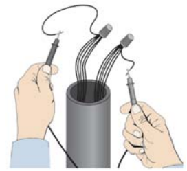
Spider Splice® junctions provide an ideal testing point.
