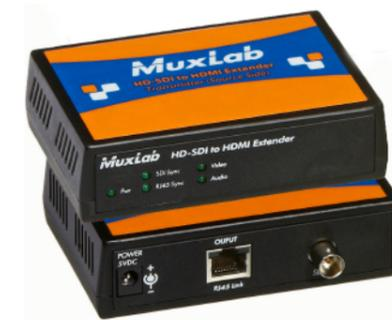
The 3G-SDI to HDMI Extender Kit (500715) converts 3G-SDI to HDMI and then transmits it up to 330ft (100m) via Cat5e/6 cable at all resolutions in a point-to-point configuration. The 3G-SDI to HDMI Extender supports transmission of up to 2.97/3.0Gbps uncompressed, un-encrypted digital video (optionally including embedded Audio and/or Time Code) within television facilities and between professional video equipment.
