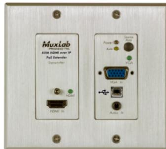
The HDMI/VGA/USB over IP PoE Wall Plate Transmitter allows HDMI, VGA and USB equipment to be connected up to 330ft (100m), with video supported at up to 4K (3840x2160) resolution @ 30Hz via one CAT5e/6 unshielded twisted pair cable in a point-to-point configuration. Point-to-multipoint and multipoint-to-multipoint configurations are also possible by connecting several Transmitters and Receivers to the same local Ethernet IP network via an Ethernet Switch.
