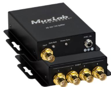
The 3G-SDI 1x4 Splitter allows one (1) 3G/HD/SD-SDI source to be distributed and amplified to up to four (4) 3G/HD/SD-SDI displays. The splitter supports up to 1080p video, including 480i (SD-SDI), 720p/1080i (HD-SDI), and 1080p (3G-SDI). The device automatically detects the 3G/HD/SD-SDI signal and re-clocks and regenerates the signal at the output for extending distances between source and displays.
