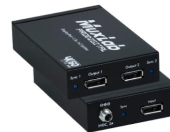
The DisplayPort 1.2a 1x2 Hub, MST (500506) is a device that allows you to extend different DisplayPort 1.2a content from one DisplayPort connector to two monitors. The hub supports video resolutions up to 4K and PCM Audio up to 7.1-Channel and up to 192 kHz sampling rate, and supports Multi-Stream Transport (MST) of up to eight streams.
