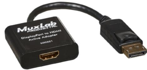
The DisplayPort to HDMI Active Adapter (500501) allows a DisplayPort source such as a PC or Laptop to be connected to an existing HDMI display or projector. The unit does not require external power to operate and comes with a lifetime warranty.
