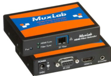
The HDMI Fiber Extender Kit (500460) allows HDMI equipment to be connected up to 1,000 ft (305m) @ 4K/30 resolution via one (1) 50/125 μm Multimode fiber cable in a point-to-point configuration. The kit comes with one (1) Transmitter and one (1) Receiver as well as an IR Emitter (500998) and IR Sensor (500999) for remote control applications.
