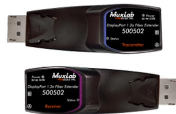
The DisplayPort 1.2a Fiber Extender Kit enables the user to transmit WQXGA (3840x2240) video at 60Hz signal up to 330ft (100m), with any form of scaling or data compression being applied to the signal. This device supports a total data throughput of 21.6Gbps (5.4Gbps per lane).
