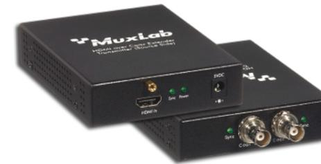
The HDMI over Coax Extender Kit (500465) allows an HDMI source to be connected to an HDMI receiver up to 250ft (76m) at 1080p resolution via one (1) coax cable in a point-to-point configuration. Furthermore, the product may be cascaded via the HDMI over Coax Receiver (500465-RX) in order to support multi-display applications.
