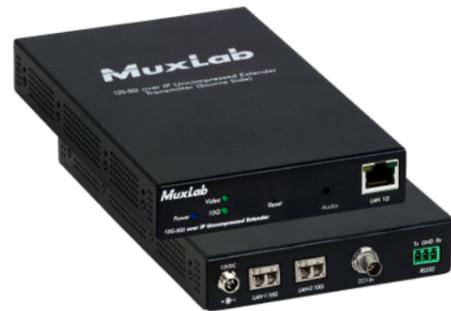
The 12G-SDI/ST2110 over IP Uncompressed Gateway Converter allows lower cost 12G-SDI equipment to be utilized in a broadcast environment and extended up to 1300ft (400m) via duplex multimode OM4 fiber with LC connectors, at up to 4K resolution @ 60Hz uncompressed, in a point-to-point configuration.
