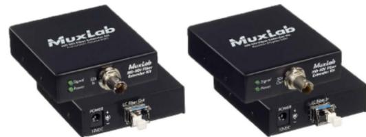
The 3G-SDI Fiber Extender Kit (500710) allows one 3G-SDI channel to be transmitted up to 19mi (30km) via one singlemode fiber in a point-to-point configuration. The 3G-SDI Fiber Extender supports transmission of up to 2.97/3.0Gbps uncompressed, un-encrypted digital video within television facilities and between professional video equipment. The 500710 includes a Hirose power cable for SDI camcorder applications and comes with a hard plastic carry case.
