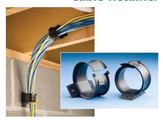
The CADDY® CATCR50 Cable Retainer is a plastic, low-voltage cable support with an easy-lock closure and an attachment base. The new cable retainer from ERICO® can be installed on walls, beams, studs, ceilings and racks – vertically or horizontally – which makes it extremely versatile. The CADDY CATCR50 support has rounded edges to avoid over-bending and kinking of cables.
