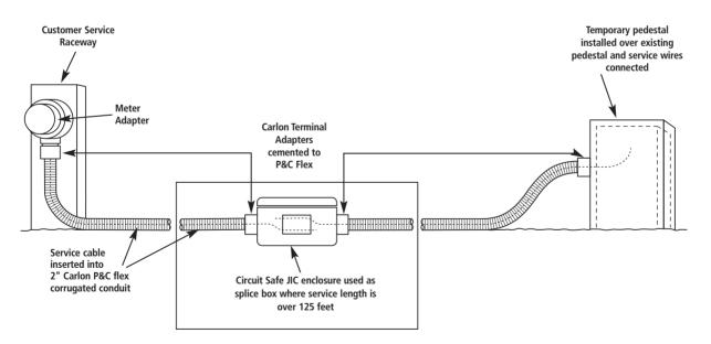
Digging up faulty cable in frozen ground can be expensive and time consuming. Use Carlon P&C Flex<sup>®</sup> from the customer service raceway to the temporary service pedestal to restore power on an interim basis. When the service length is over 250 feet, use a splice box and an additional length of P&C Flex<sup>®</sup> Nonmetallic Corrugated Conduit.
