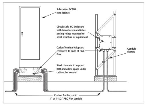
Carlon P&C Flex<sup>®</sup> Nonmetallic Corrugated Conduit protects control cables in supervisory control and data acquisition equipment (SCADA) in distribution substations. Flexibility provides maximum utilization of equipment.
