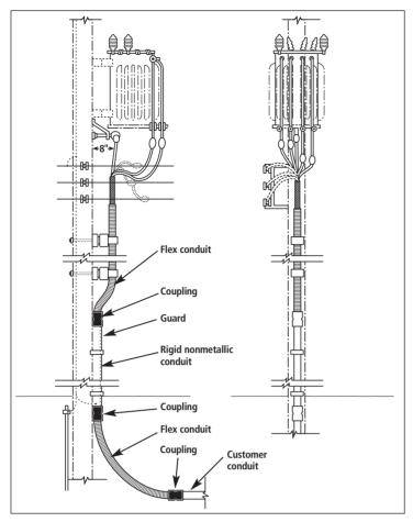
P&C Flex<sup>®</sup> conduit is flexible. Carlon P&C Flex<sup>®</sup> Nonmetallic Corrugated Conduit is used to transition from Carlon P&C<sup>®</sup> Duct Type DB. Despite equipment being mounted away from the pole, P&C Flex<sup>®</sup> conduit remains flush to the pole.
