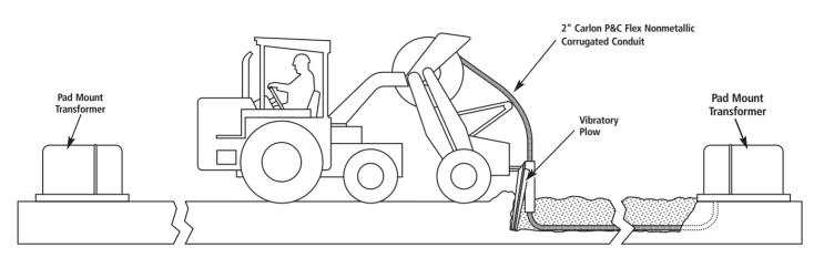
In single phase underground primary systems, lower the cost of direct buried and standard conduit systems by installing P&C Flex<sup>®</sup> Nonmetallic Corrugated Conduit with a vibratory plow.
